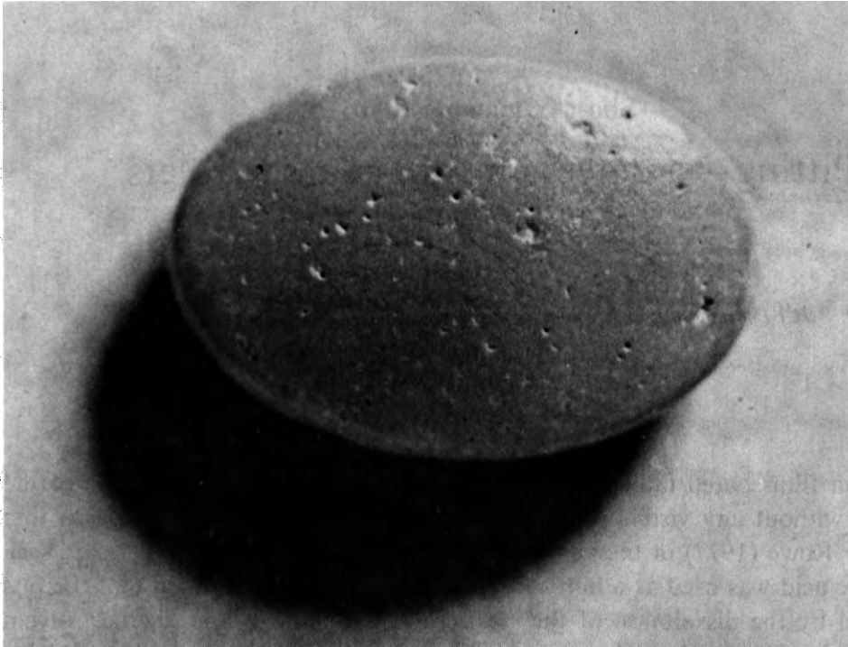
Fig. 1. A film-coated tablet showing pitting in the surface of the tablet core.
